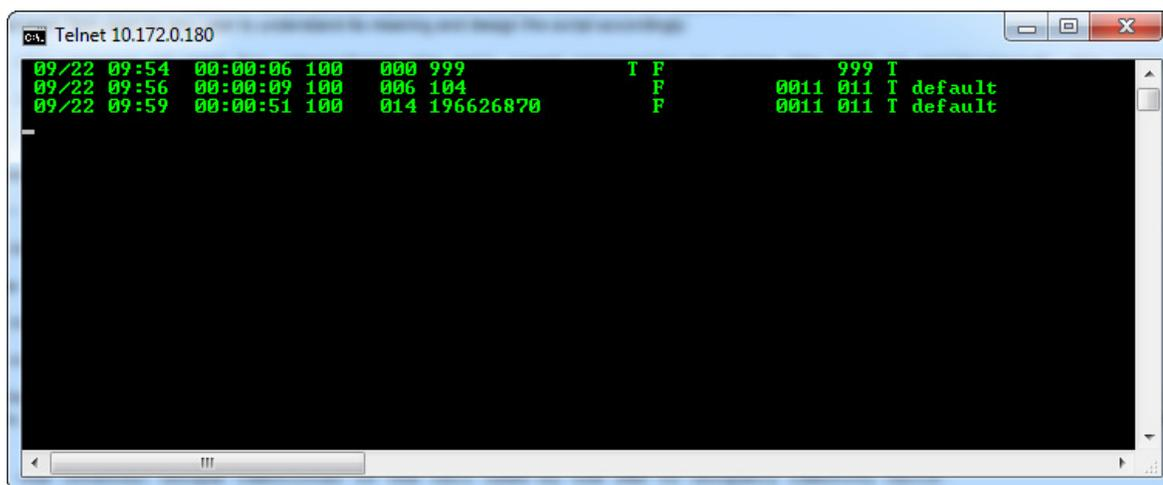
A screenshot of a Telnet window titled "Telnet 10.172.0.180". The window shows three lines of SMDR output in green text on a black background. The first line is "09/22 09:54 00:00:06 100 000 999 I F 999 I". The second line is "09/22 09:56 00:00:09 100 006 104 F 0011 011 I default". The third line is "09/22 09:59 00:00:51 100 014 196626870 F 0011 011 I default".
