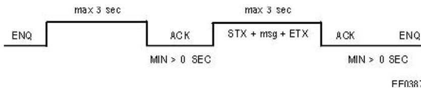
The maximum time to wait for the ACK after a STX + msg + ETX transmission is 3 seconds.
